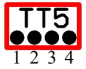
Tetrodes 5-8 are laid out according to the diagram to the left, when looking at the TT# label right side up. Notice they are different than Tetrodes 1-4.
