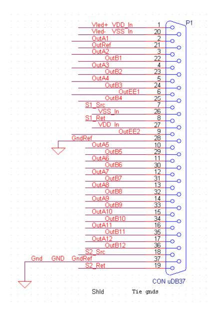
Figure 4-1: Pin Out of the uD37 Tether Connector
