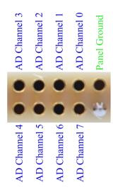
9 Pin Female Nano Omnetics Connector **Figure 1 HS-8-CNR-MDR50 Input Pinout**
