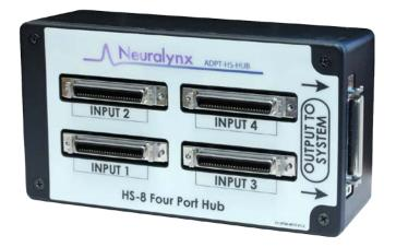
The ADPT-HS-HUB is an adapter that allows up to 4 HS-8s to interface with a single MDR-50 input connector on the Digital Lynx Data Acquisition System or Cheetah 32 Data Acquisition System.
