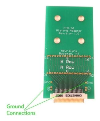
**Figure 4-1 Plating Adapter Ground Locations**
