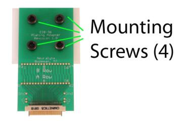
Figure 3-1 Mounting Screws (4)
