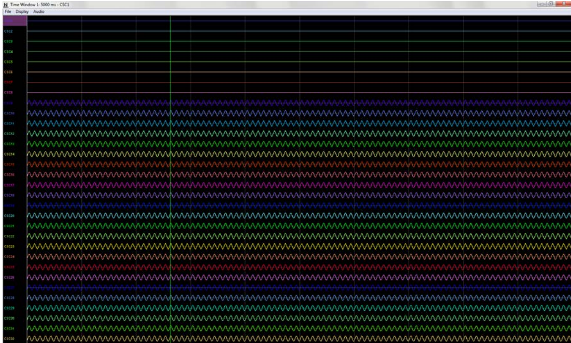
Figure 4-4 Bank 2, 3 and 4 Switches Up. Bank 1 and Reference Switches Down. Switch the Bank 2 Switch to the Ground Position (Down). Observe the 32 CSCs. CSCs 1-16 should now be flatlined while CSCs 17-32 still show a reduced (roughly 1mV PP ) version of the Minirator output. Refer to the figure below.
