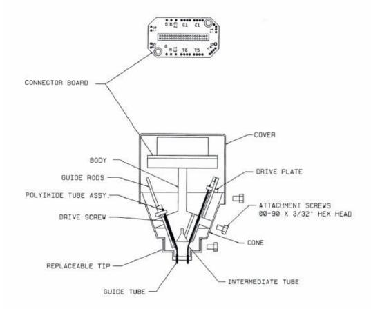
Figure 10.1 Microdrive Parts Identifier
