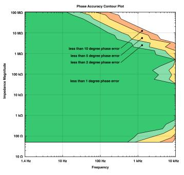
Accuracy contour plots were based on impedance measurements of fixed resistors between 51 Ω and 100 MΩ. Magnitude and phase accuracy assumed ideal resistor behavior. Magnitude accuracy was evaluated by comparing the Imp impedance magnitude measurements to the compensated impedance magnitude measurements at 1 Hz of a Gamry Reference 600 potentiostat. Phase accuracy was evaluated by comparing the Imp impedance phase measurements to 0 degree phase.
